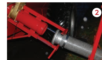
The hose slides into the connection fork.
