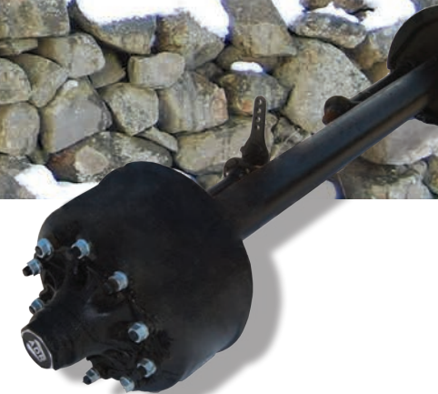
10 Stud 420 x 180 S - Cam Commercial Axle
