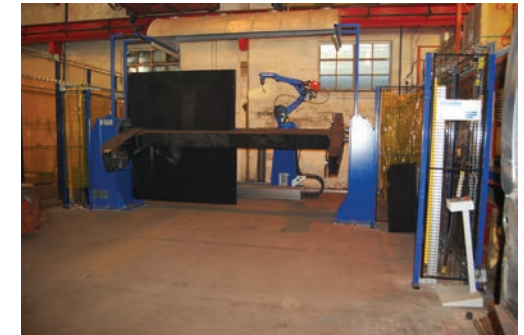
Above: New Robotic Welding Cells
