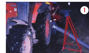
The tractor draws up to the hose with the connection fork extended.
