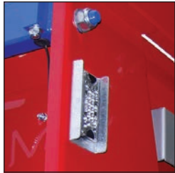
High Level LED Lights
