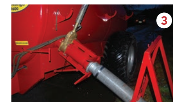
The hose is pulled tight against the coupling to create an air tight seal.
